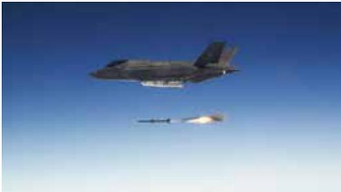
In a rigorous testing environment encompassing 42 WDAs, we certified the F-35 for the AIM-120, AIM-9X, ASRAAM, Paveway IV, SDB, GBU-12, GBU-31, JDAM, and JSOW.
