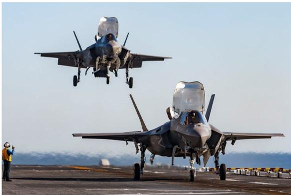
After three weeks on board, and just in time for Thanksgiving, our PAX River test team completed DT-III for the F-35B. Overall, they accomplished 60 flights, 128 vertical landings, 126 short takeoffs, two vertical takeoffs, and expanded the F-35B's shipboard operating envelope to full operational capability for the U.S. Marine Corps.
